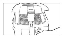
In the upper position the lid will lift out of its guides at the back for easy cleaning. To
